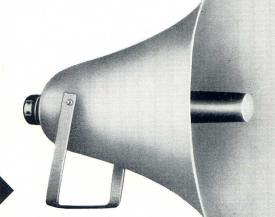
Standard reflex horn speaker for medium distance projection of speech and incidental music, for use where the advantage of smaller overall dimensions than the PA130 is desirable. Flare diameter, 2' 2½"; length with unit, 2'.
