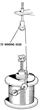
wire to remain threaded when the winding is stopped suddenly. The remaining operation is to adjust the Top Friction Disc, Item 15, to give the desired tension according to the wire being de-reeled. To do this the Lower Hand Nut, Item 9, is screwed in a clockwise or anti-clockwise direction and when set is locked by the Upper Hand Nut.
