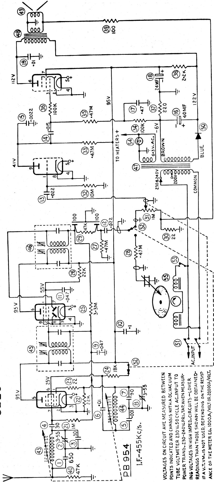
VOLTAGES ON CIRCUIT ARE MEASURED BETWEEN POINTS INDICATED AND CHASSIS WITH A DC VACUUM TUBE VOLTMETER 230V-5 CYCLE AC INPUT TO POWER TRANS. 230-240V PRI. TAP. WHEN MEASURING VOLTAGES IN HIGH IMPED. CIRCUITS → LOWER READINGS THAN THOSE SHOWN WILL BE OBTAINED IF A V.T.V.M. IS NOT USED, DEPENDING ON THE RESISTANCE OF THE METER E.G. 1000Ω/VOLT OR 2000Ω/VOLT.
