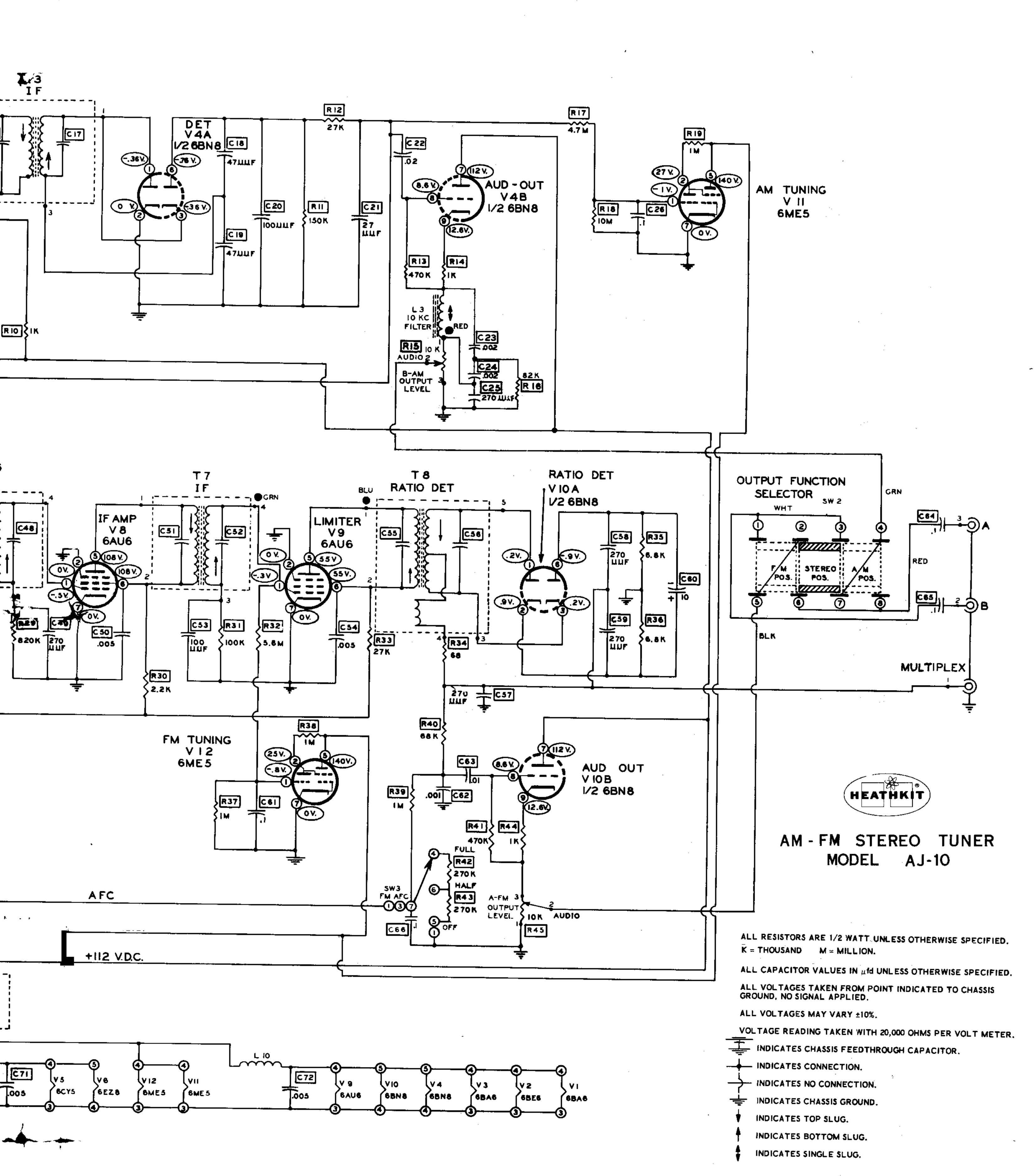
Schematic has been corrected to show B+ supply for indicator tubes V11 and V12 coming from the +112vdc bus, right end of R47 as indicated in assembly instructions (page36), rather than from +140vdc at the left end of R46.
