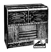
This model is a six-valve A.C. mains-operated medium-wave and bandspread short-wave console radiogram, incorporating a three-speed automatic record changer.
