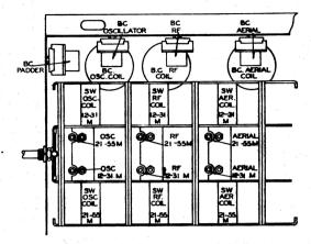
IF Alignment: Set the oscillator to 392 KC, and comment to the grid of the CKl valve. Turn the volume control full on, the tone control to the right, and the wave change switch to the Broadcast band (extreme anti-clockwise position). Adjust the four trimmers on the two IF transformers for maximum gain. Sensitivity should be approximately 100 microvolts.
