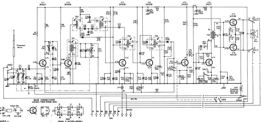
Voltages measured with no signal input with a 20,000 ohm volt meter.
