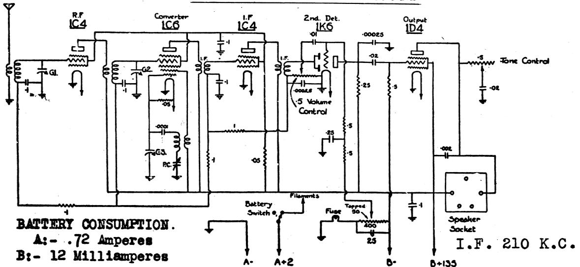
**MODEL 855.** - 5 Valve Broadcast with heavy duty "B" batteries and one 2 volt "A", in standard upright or standard console cabinet, fitted with automatic volume control, 8" edgelit dial and 10" dynamic speaker.
