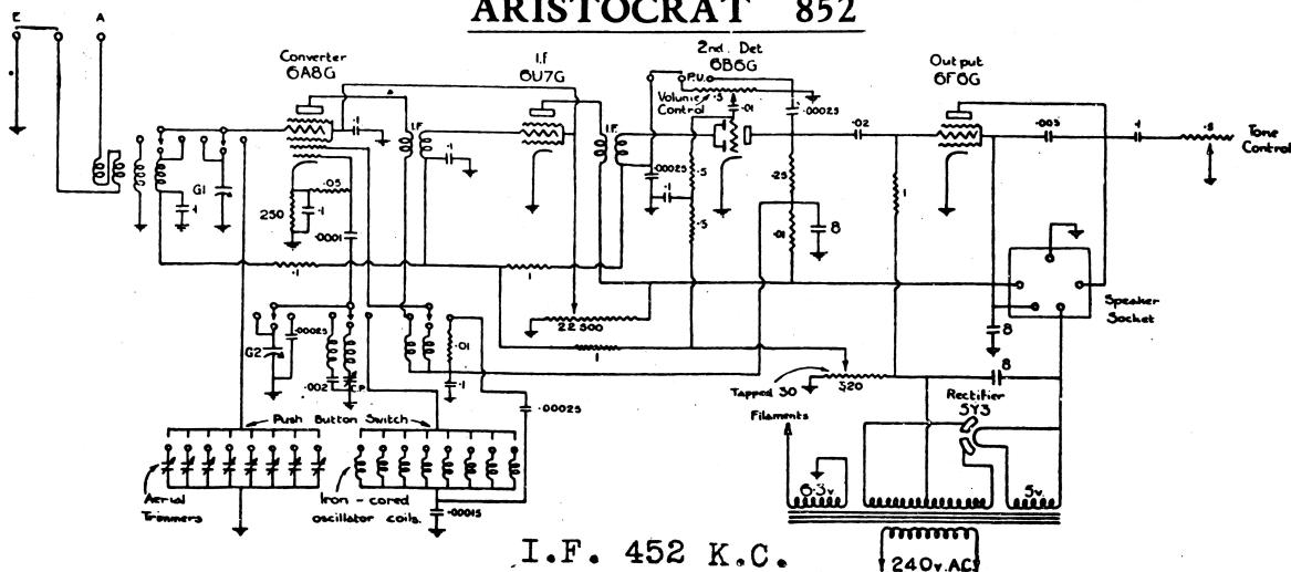
MODEL 852. - 5 Valve Dual Wave, in standard upright or standard console cabinet, fitted with AUTO-
