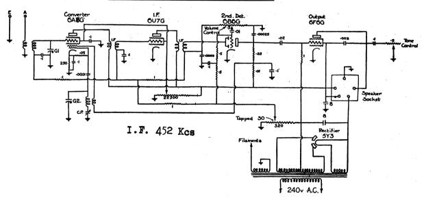
MODEL 850. - 5 Valve Broadcast, in standard upright or standard console cabinet, fitted with automatic volume control, 8" edgelit dial tone control and 8" speaker.
