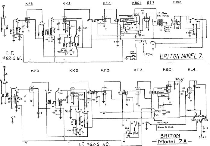
Briton models "7" and "7A" are both six-valve dual-wave battery-operated console receivers, each using a 10-inch permag. loudspeaker. Model "7" originally was introduced as a "de luxe" version of model "6," but was discontinued after serial No. 25 in favour of model "7A." This last follows the design of model "6" fairly closely, but differs in some important features such as the use of permeability-tuned I.F. transformers and two I.F. amplifier stages.
