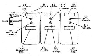
The trimmer capacitors on the coil assembly and intermediate frequency Transformers (tuned to 392 K.C.) are adjusted and sealed at the factory. These adjustments should on no account be touched or seals broken unless a calibrated oscillator and indicating instrument are available, whereby such adjustments can be successfully carried out.
