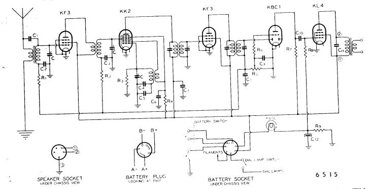
The two receivers shown above normally are operated from a 2-volt accumulator and 3-45 v. "B" batteries. With the addition of a Philips' type "148" vibrator H.T. unit, either may be completely operated from a 6-volt accumulator. Also, the filament drain is low enough to permit of using "air-cell" A supply. Further details are given opposite.
