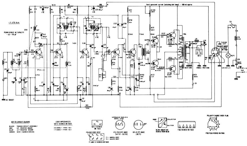
NOTE: 0-0 INDICATES INTERCONNECTING LINKS, MAIN PRINTED PANEL TO SUB-ASSEMBLIES
