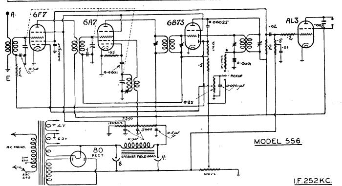
Stromberg-Carlson models "536" and "556" are "dual-wave" and "broadcast" versions of one basic circuit arrangement; both versions are illustrated for convenience of reference. These receivers are of the console type and are fitted with 8-inch, 1,000 ohms field, loud-speakers. Four controls are fitted to model "536," these being for volume, tuning, tone (continuous) and wave-change while three controls are fitted to model "556"—the wave-change switch being omitted.
