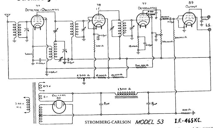
Stromberg-Carlson model "53" is a five-valve receiver designed for broadcast coverage and operation from 200-260 v., A.C., supply. This receiver is of the mantel type and is fitted with two controls, these being for volume ("R.F." type) and tuning. The loudspeaker has a field-coil resistance of 1,300 ohms. This model was marketed during 1933.
