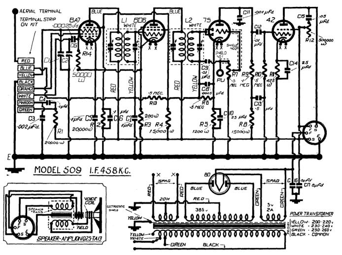
Lekmek model "509" is a five-valve receiver designed for dual-wave coverage and operation from 200-260 volts A.C. mains. This receiver is of the console type and is fitted with four controls—volume, tuning, wave-change, and tone (continuous). The loudspeaker is an sinch unit with a field resistance of 2,500.
