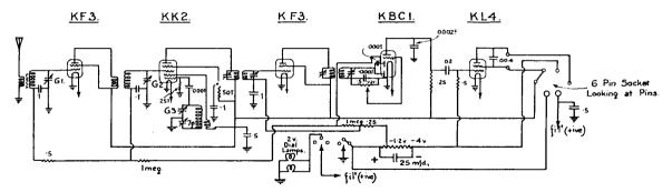
Intermediate Frequency-462.5 kC. 8-inch, permag. loudspeaker.
