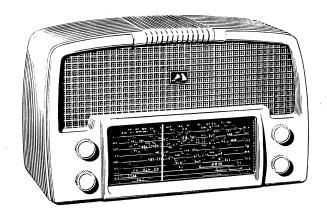
This model is a five-valve A.C. mains-operated, medium-wave and bandspread short-wave table receiver.
