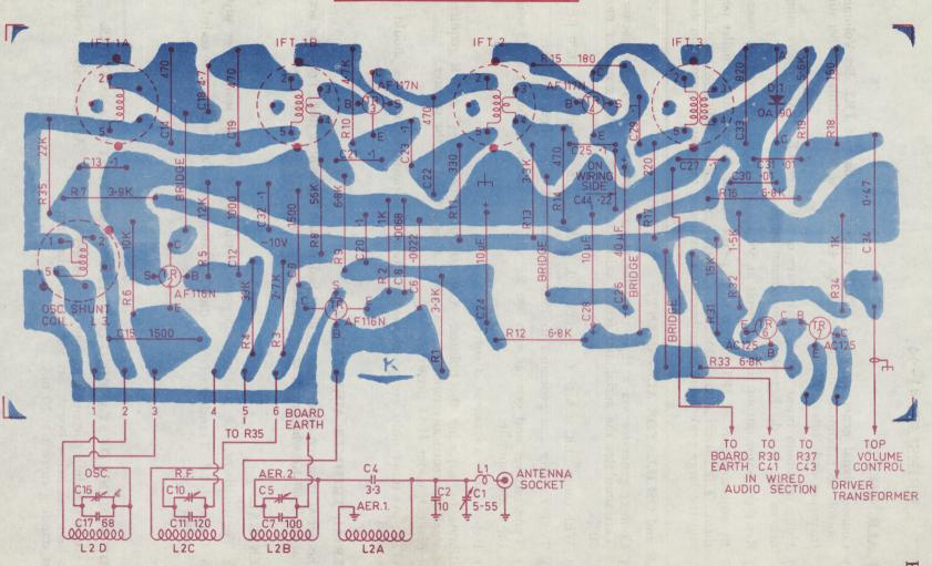
VIEW FROM CONDUCTOR SIDE OF PRINTED WIRING BOARD
