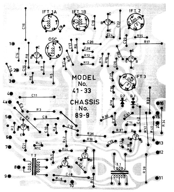
VIEW FROM CONDUCTOR SIDE OF PRINTED BOARD © EXTERNAL CONNECTIONS TO P.W. BOARD AS SHOWN ON CIRCUIT DIAGRAM.
