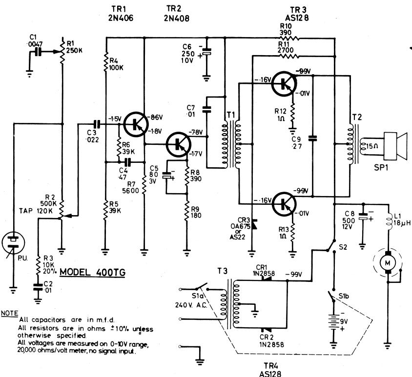
Power Supply: Mains operation: 230-250 volts AC 50 c.p.s.
