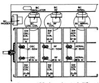
IF Alignment: Set the oscillator to 392 KC and connect to the grid of the KK2 valve. Turn the volume and tone controls full on, and the wave change switch to the Broadcast band (extreme anti-clockwise position). Adjust the four trimmers on the two IF transformers for maximum gain.
