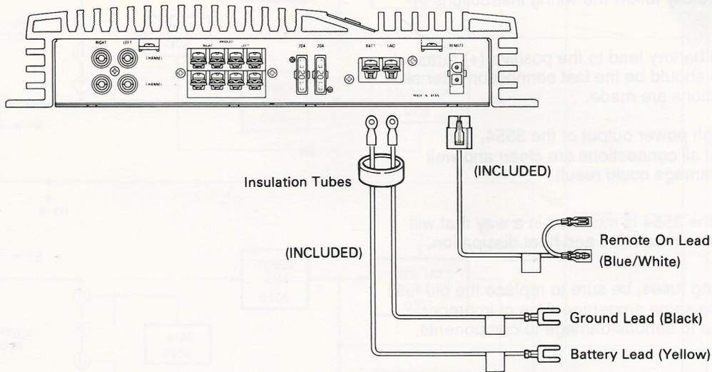
Before making connections, be sure to turn the power off to all audio components. Insulation tubes for the speaker leads and the power supply leads are supplied with the 3554, route the speaker leads and the power supply leads separately through these tubes.
