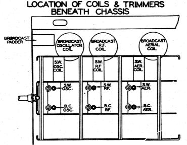
IF Alignment: Set the oscillator to 392 KC, and connect to the grid of the KK2 valve. Turn the volume and tone controls full on, and the wave change switch to the Broadcast band (extreme anti-clockwise position). Adjust the four trimmers on the two IF transformers for maximum gain.
