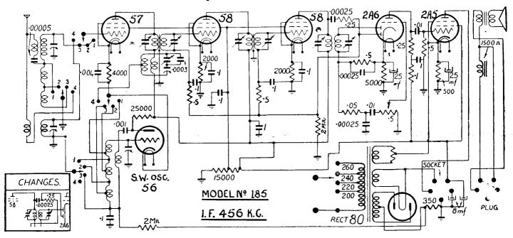
Genalex model "185" is a seven-valve receiver designed for "all-wave" coverage (four bands—13/27, 25/50, 48/100 metres, and broadcast) and operation from 200-260 volts A.C. mains. This receiver is of the console type and is fitted with four controls, these being for volume, tuning, wave-change and aerial circuit trimming (on short-wave bands only). The loudspeaker fitted is an eight-inch unit with a field-coil resistance of 1,500 ohms. This model was marketed during 1934.
