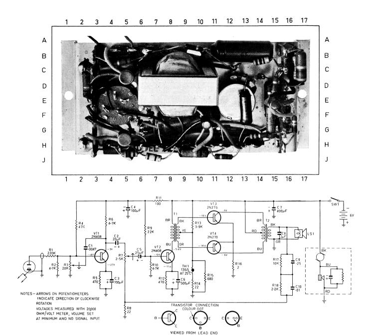
Note: C4 is now a  $500\mu\text{F}$  18 VW Electrolytic. Code No. 229853.
