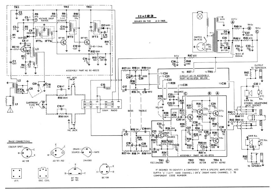
SERVICE PRECAUTIONS, TRANSISTOR A.D.161 — DO NOT (ACCIDENTLY) SHORT-CIRCUIT THE COVER, MOUNTING SCREWS, OR NUTS TO CHASSIS, NOR TO BASE, OR EMITTER LEADS.
