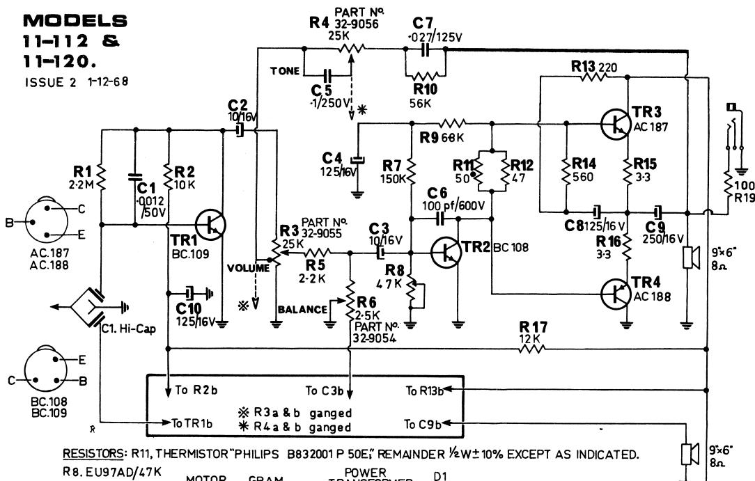
**RESISTORS:** R11, THERMISTOR "PHILIPS B832001 P 50E"; REMAINDER  $\frac{1}{2}W \pm 10\%$  EXCEPT AS INDICATED.
