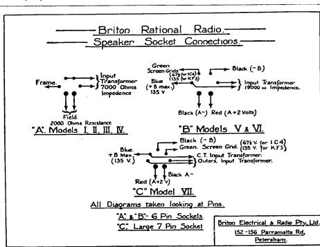
Above are shown the loudspeaker and loudspeaker-battery plug connections used with "Briton" models 1 to 7A. inclusive. Since the above block was made, Briton's address has been changed to 369 Kent Street, Sydney.
