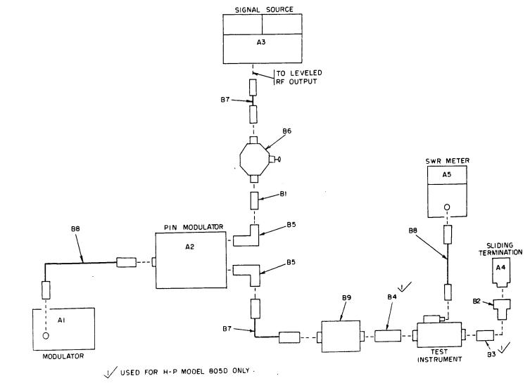
Figure 1. Residual VSWR - equipment setup for Hewlett-Packard Models 805() and IM-92()/U.
