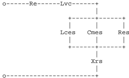
Now, the relative values of these components depends upon the magnitudes of the physical values times a transformation factor. That transformation factor is the electromagnetic transduction factor, proportional to the Bl product (the product of the length of the wire l immersed in the magnetic field B), measured in N/A (or T/M, if you will). So, IF we know the magnitudes of the physical components, we can easily calculate their electrical equivalents:
